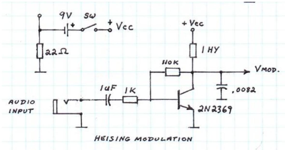
This QRP (low powered) broadcast transmitter was designed and built by Reed, W2CQH, to use at the SARS monthly meetings for those who brought in broadcast radios and wanted to show off how well they worked. The building where we meet is steel framed so reception is marginal at best, plus we can play our own selections of favorite music. I will say the fidelity is very good for such a simple device and the Heising modulation works quit well and seems to boost the effective power of the device.
