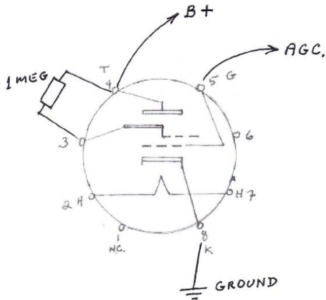
How is the Cat’s eye constructed? Here’s an outline of its structure:
