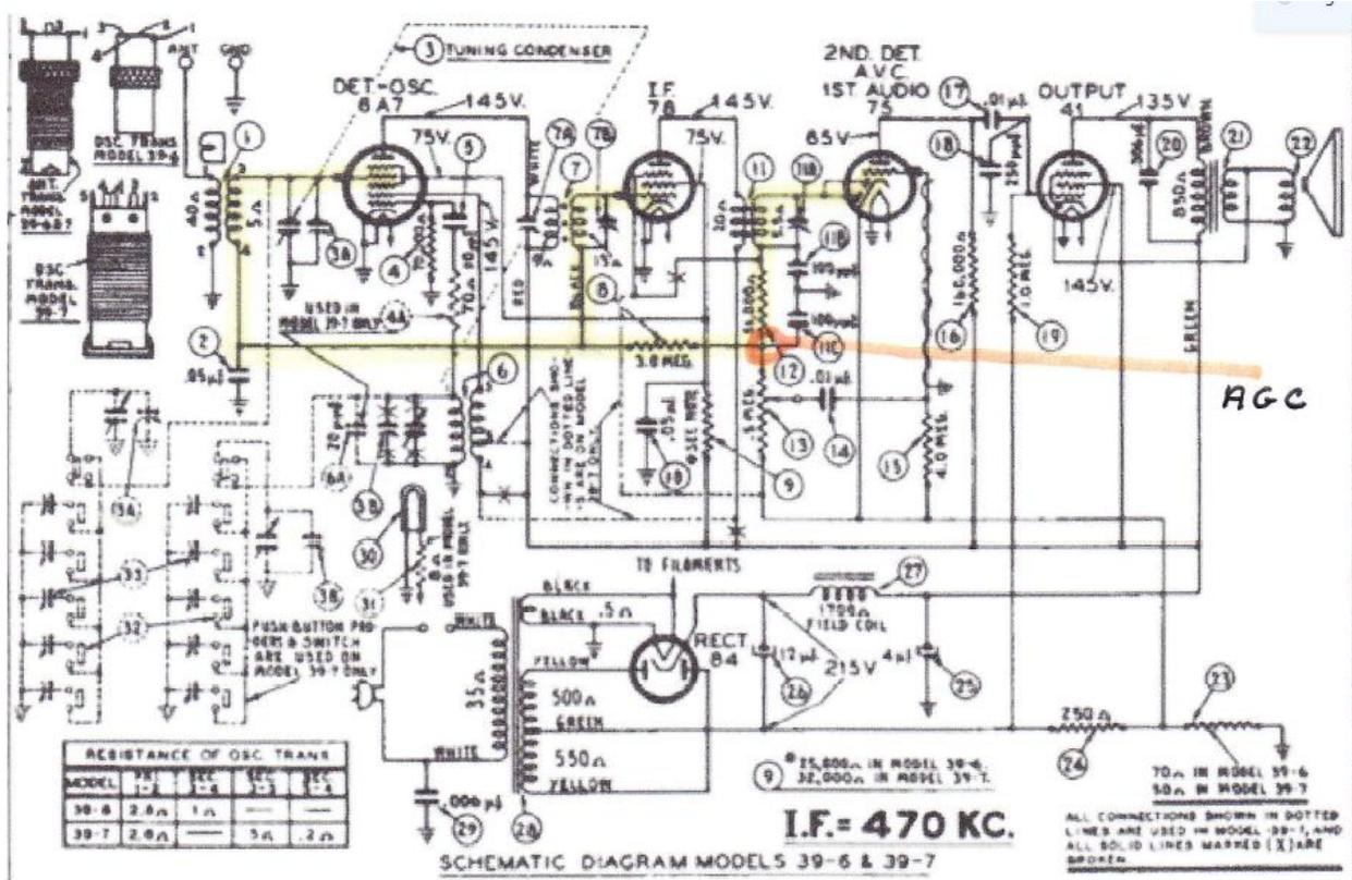
And below is a detail of the detector/AGC where you would connect to the grid of the Cat's Eye.
