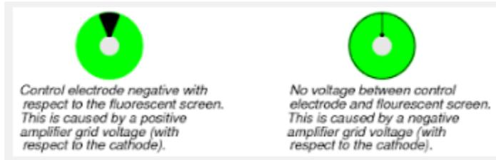
As the AGC swings negative when you tune in a strong station, the tube will appear to close up as shown on the right.
