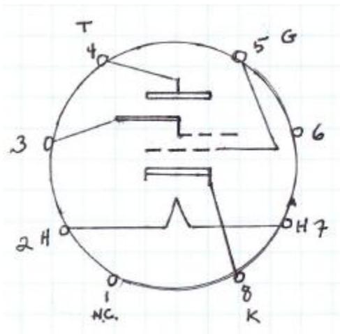
Note that the heater voltage is pin 2 and 7. You should be able to get this from your radio. If you have only a 6.3 volt supply, never fear. You can easily make a voltage doubler circuit. It runs fine on 12 volts DC.
